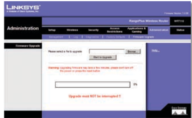
Administration &gt; Firmware Upgrade
